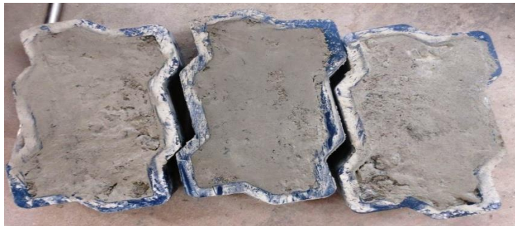
Figure 2. Geopolymer concrete cast in paver moulds
