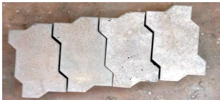
Figure 3. Geopolymer concrete pavers after demoulding.
