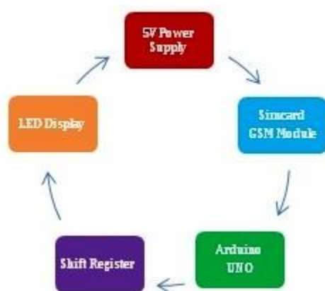
Figure 1: Proposed block diagram of Wireless LED Notice Board
