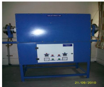
Fig.3. Horizontal Tubular Furnace used for annealing the samples
