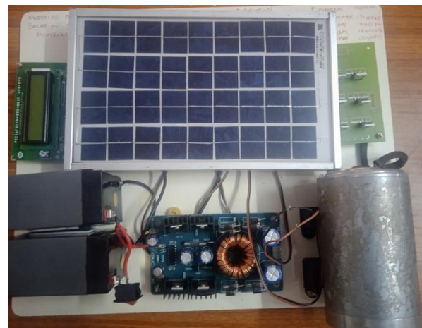
Figure 3: A laboratory prototype of IoT based Smart Solar based Industrial Motor
