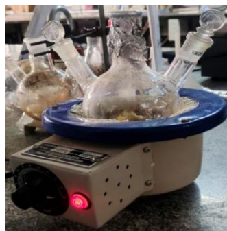
Fig 3: Hydrolysis process set-up
