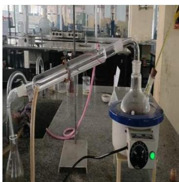
Fig. 7. Distillation process set-up
