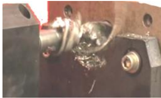
Figure 1 Typical example of Fin breakage
